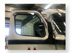
1. Weather Shield Slim Fit Driver side - Q PPH DT001SLD Passenger side - Q PPH DT001SLP
